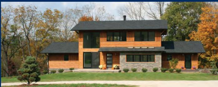
The design of the new home embraced the large, low-pitched bracketed overhangs seen on the other camp buildings (below). Large expanses of glass were important in order to take advantage of views over the bluff to the river behind the home.
